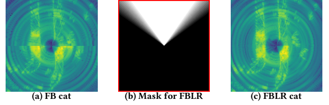
Figure 3: Images representing: (a) Radar image after Front-Back (FB) concatenation, (b) Mask for Front-Back-Left-Right (FBLR) concatenation, (c) Radar image after concatenation of all four views.
