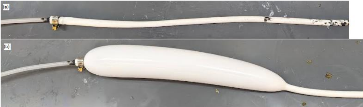
Figure 3.3.1 Bladder for tube fabrication. (a) deflated, (b) inflated.
