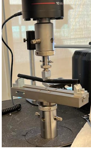
Figure 3.4.1 CFRP tube flexural strength test setup.
