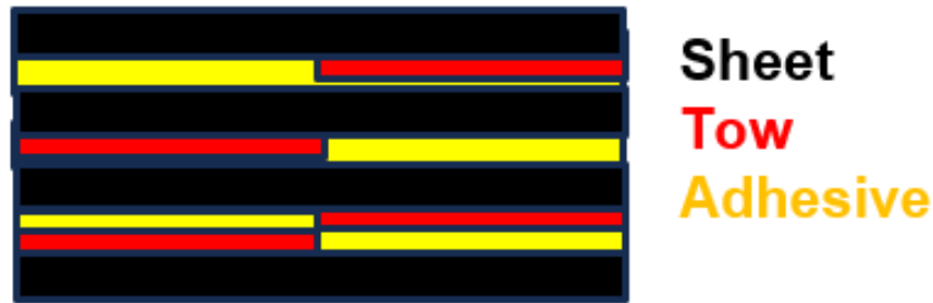
Figure 3.5.1 Laminate layup for short beam shear test.
