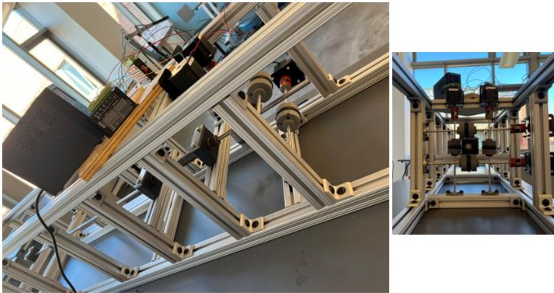
Figure 6.2.1 Partially built pultrusion machine to fabricate tubes.
