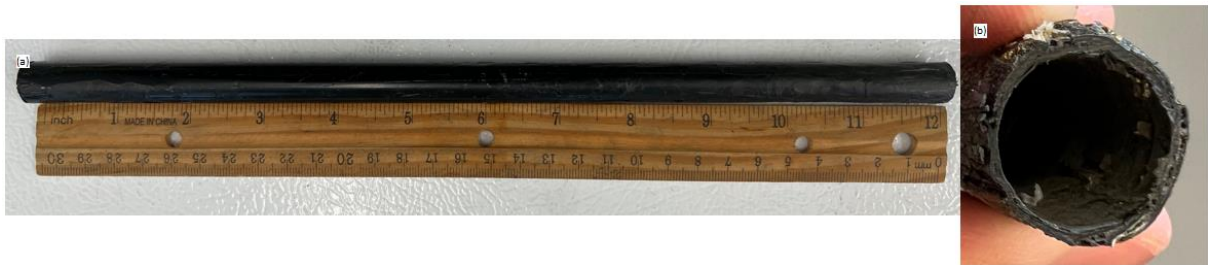
Figure 3.3.5 (a) Fully cured tube and (b) the tube cross section.
