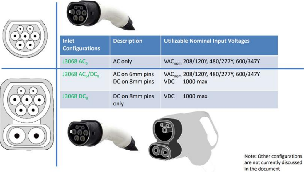
Figure 2.4. Part of Specifications for J3068
