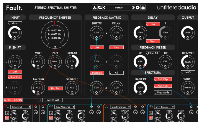
Figure 5.3: Fault interface, with expandable modulation system visible.
