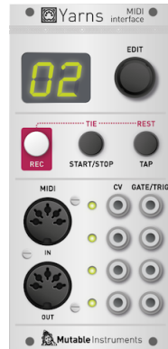
Figure 3.5: Mutable Instruments Yarns. This module converts MIDI messages into control voltages and gates.
