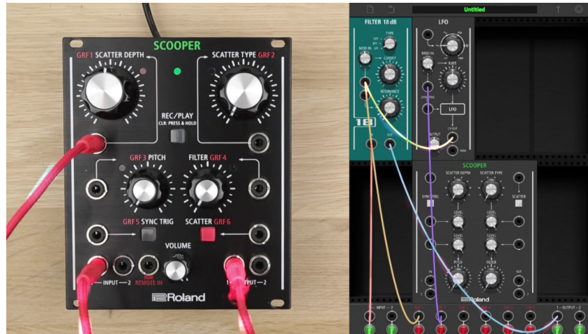
Figure 6.21: Roland Scooper, shown next to the Roland Modular Customizer. Here, the base effect is combined with an animated filter.
