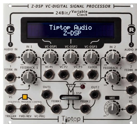
Figure 2.4: Tiptop Audio Z-DSP. Note the cartridge reader on the front for loading different algorithms.
