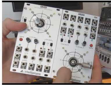
Figure 3.3: Intellijel Planar, here demonstrated with two different faceplates. The module can be inverted to help avoid cables from physically interfering with the user’s range of motion.
