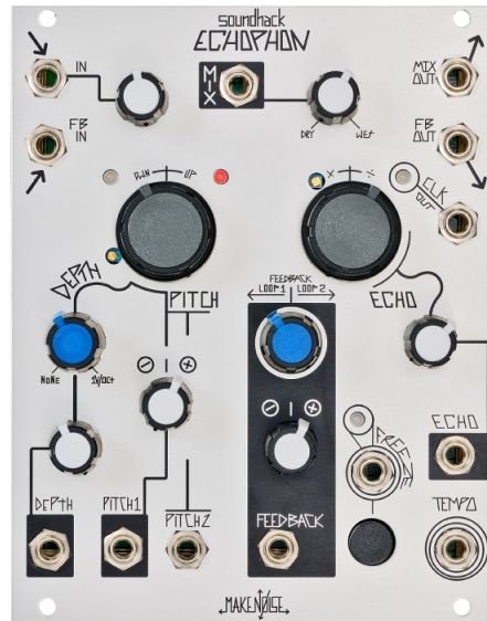
Figure 2.7: Make Noise Echophon. Note the CLK OUT jack in the top right.
