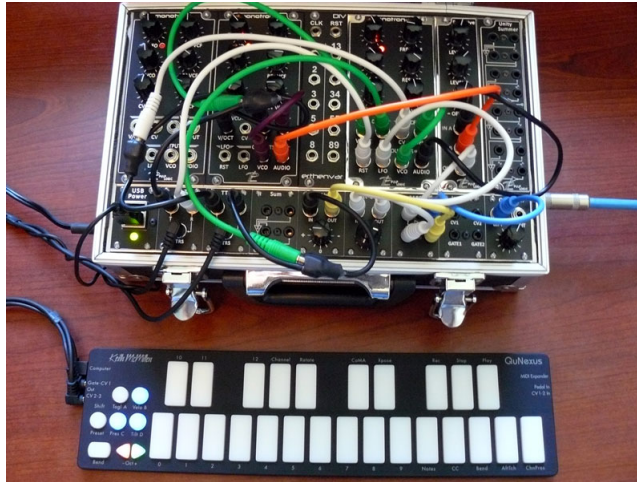
Figure 3.4: Keith McMillen QuNexus, here interfacing directly with a Eurorack system via CV outputs. The QuNexus can connect to a computer via USB and provide MIDI-over-USB.
