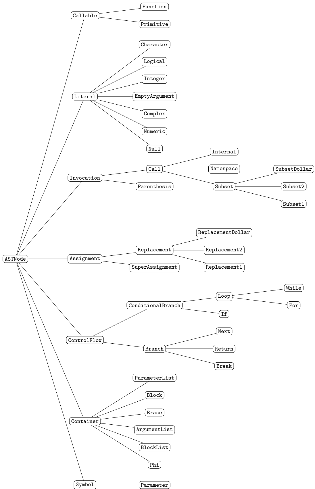
Figure 1.2: The hierarchy of classes provided by the rstatic package to represent expressions.
