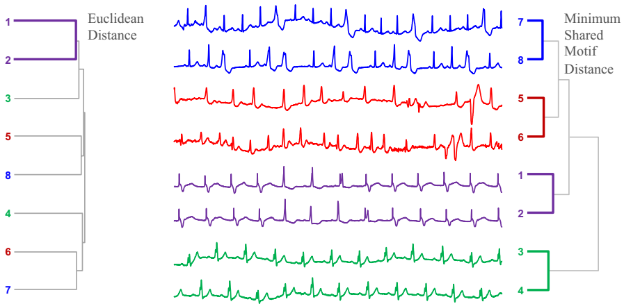
Fig. 8 (Left) Eight 10-s snippets of time series, from four individuals, clustered using Euclidean distance single-linkage hierarchical clustering. (Right) The same snippets clustered using a Matrix Profile based distance measure
