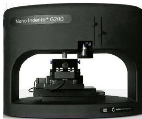
Figure 2.10 Schematic photograph of a G200 Agilent Nanoindenter similar to the one used at the University of Oxford for dynamic nanoindentation (CSM).
