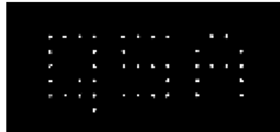
Two-dimensional arrays of individually focused laser beams arranged images of 42 atoms (Credit: Harvard University)
