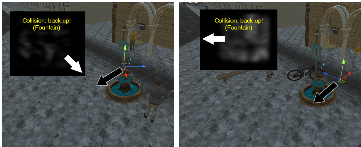
Figure 6.4: To avoid participants walking through virtual objects, they were forced to ‘back up’ when a collision was detected. To back up, they had to move 0.25 meters in the negative z-direction. To accomplish this, a UI element would appear informing the participant of the collision. There was text stating “Collision, backup!” along with the name of the object collided with (for example ‘Person, walking’ if they collided with a moving person). Additionally, there was an arrow telling them which direction to back up in. In this figure, the participant (represented by the three colored arrows with blue being forward) has approached the fountain from two separate directions. In the left figure, they approached from the southwest, and were told they needed to go back and to the right to complete their “Back-up”. In the right figure, the participant approached from the east and was told they needed to go directly left to complete their “Back-up”. In both cases, the participant is simply being told to go south (black arrow), back towards the starting location.
