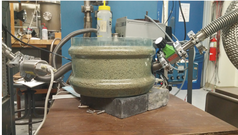
Figure 3.4: Sending the pump line through a large amount of sand was enough to dampen out the vibrations from the pumps.
