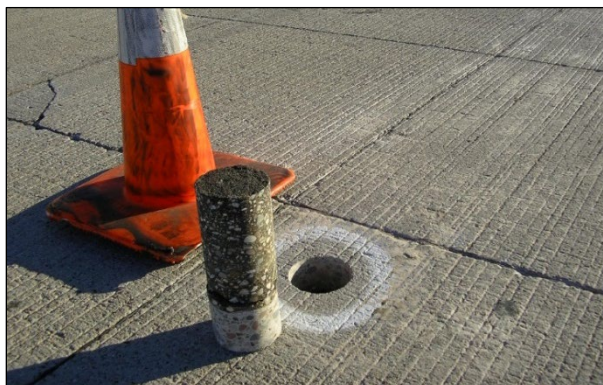
Figure 3.43: Core of concrete with asphalt base (core is upside down in photograph).
