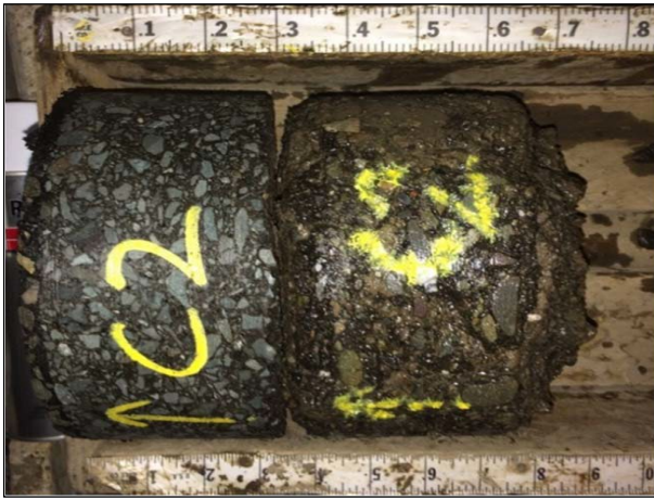
Figure 3.46: Layer debonding and moisture damage at debonded interface.
