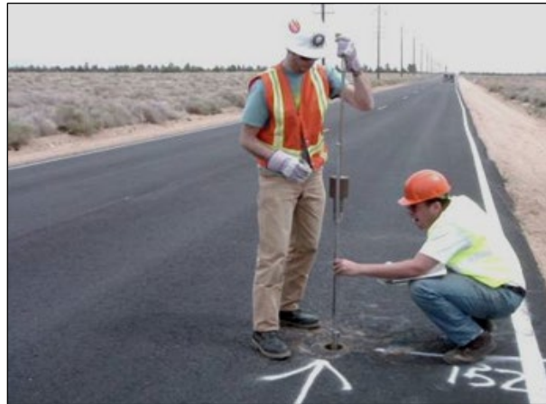
Figure 3.48: DCP testing (manual DCP).
