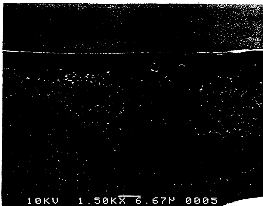
Figure 3(d) Oxide scale formed on the bulk specimen
