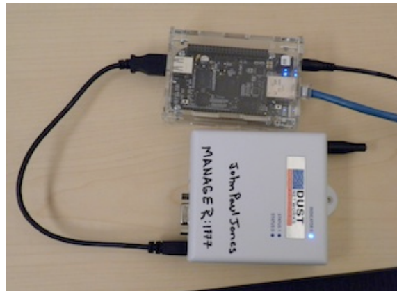
Figure 4. Manager mote and embedded computer.
