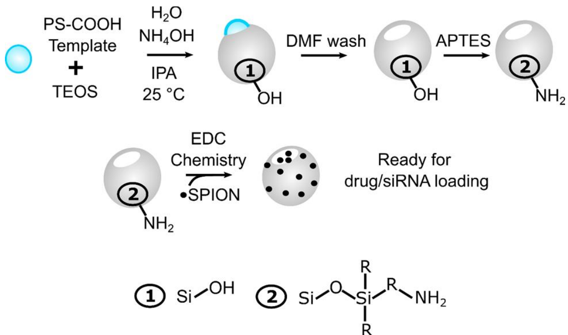
Figure 6.1. Schematic showing synthesis of magnetic NBs. Schematic shows that NBs are first synthesized with poly condensation of tetraethyl orthosilicate (TEOS) around a 100 nm polystyrene (PS) template at room temperature. Post synthesis, the NBs are purified and incubated with dimethyl formamide (DMF) at 60°C for 3 hrs, followed by silanization with 3-aminopropyl triethoxysilane (APTES). Amine functionalized NBs are conjugated with 15 nm superparamagnetic iron oxide nanoparticles (SPION) using EDC crosslinker chemistry. For more details refer to methods.
