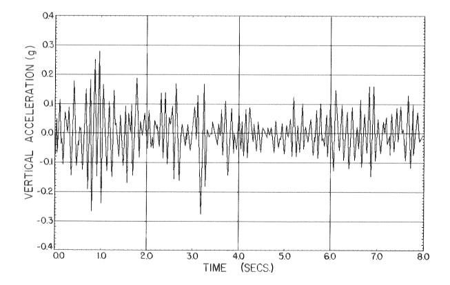
Fig. 3 - GROUND ACCELERATIONS EL CENTRO EARTHQUAKE, MAY 18, 1940
