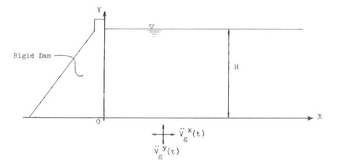
The dynamic water pressure p = p(x,y,t) is related to the gradients of displacement:
