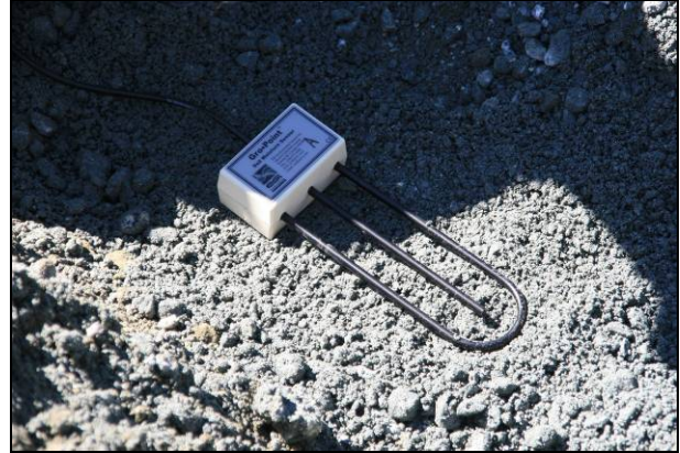
Figure 2.10: Installation of moisture sensors.
