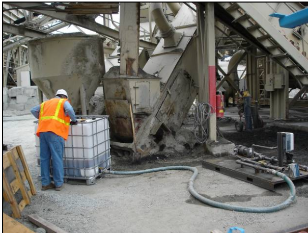
Figure 2.22: Plant modifications for admixtures.
