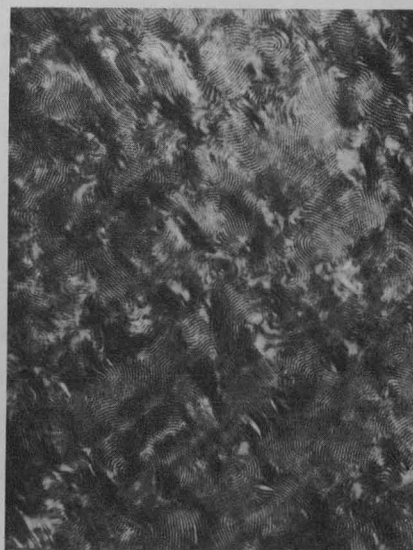
Fig. 1. Transmission electron micrograph of a block copolymer consisting of polystyrene and polybutadiene blocks (SBS).
