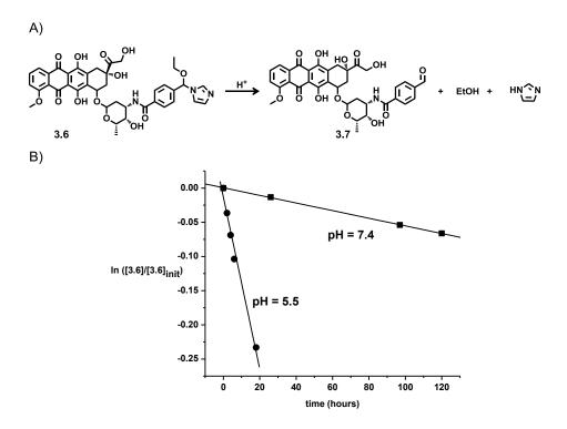
Figure 3.3 A) The schematic for hydrolysis of 3.6. B) Hydrolysis of **3.6** at 37 °C at pH 5.5 and pH 7.4, monitored at 470 nm using HPLC methods.
