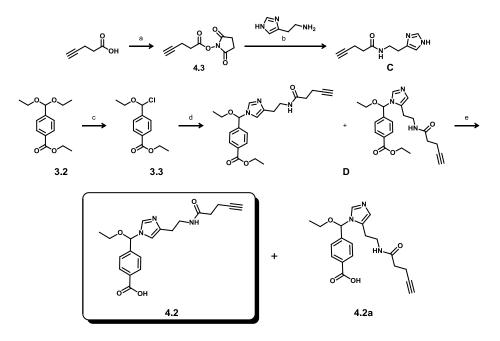
Figure 4.3 Synthetic scheme for bifunctional crosslinker para-Nethoxybenzylimidazole-alkyne-carboxylic acid 4.2. Reagents: a) NHS, EDC, DCM; b) 0.1 M HEPES buffer 53 % yield; c) acetyl chloride, thionyl chloride; d) B, NaH, in THF, 21% yield over two steps; e) lithium hydroxide, water and THF.
