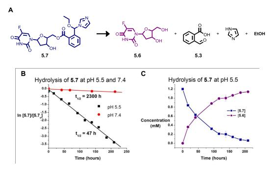
*Figure 5.7 A)* Schematic of 5.7 hydrolysis B) Hydrolysis of 5.7 and pH 5.5 and 7.4. C) Concentration of 5.7 and 5.6 over time as 5.7 hydrolyzes at pH 5.5.
