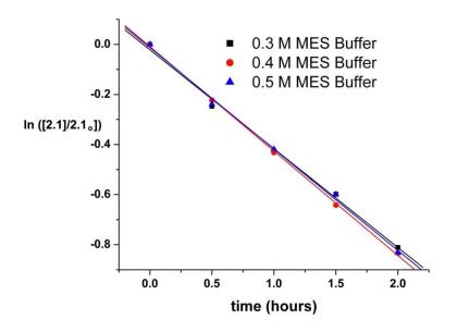
Figure 2.4 The dependence of the concentration of 2-[N-morpholino]ethanesulfonic acid (MES) buffer on the rates of hydrolysis of N-ethoxybenzylimidazole 2.1.
