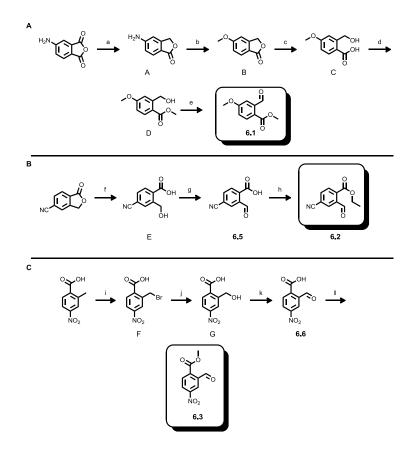
Figure 6.1 Schematic of the synthesis of 6.1, 6.2 and 6.3. A) Synthesis of 6.1. Reagents: a) Zn, sodium hydroxide in water at 0 °C, 96% yield b) water and concentrated HCl, NaNO<sub>2</sub>, MeOH c) potassium hydroxide, MeOH 60% yield, d) MeI, sodium carbonate, DMF, e) manganese oxide, THF, 55% yield. B) Synthesis of 6.2 f) LiOH, THF, water, 98% yield, g) manganese oxide, THF, reflux 32% yield, h) Etl, potassium carbonate, DMF, 92% yield.
