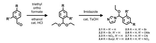
*Figure 2.5 General procedure for the synthesis of N-ethoxybenzylimidazoles (NEBIs) 2.1-2.8 from the corresponding benzaldehydes.*
