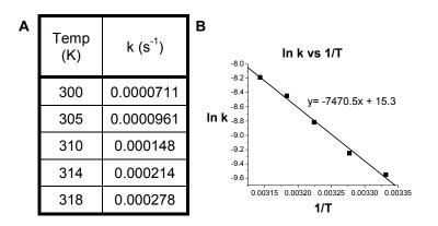
Figure 2.10 A) The rate of hydrolysis for 2.1 at pH 5.5 and varying temperatures. B) The Eyring Plot used to relate temperature and rate. The slope from this graph allowed for calculation of  $\Delta H^{\dagger}$ , while the y-intercept may be used to calculate  $\Delta S^{\dagger}$ .
