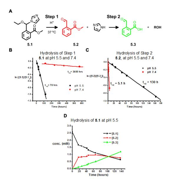
Figure 5.3 A) A schematic of the hydrolysis of **5.1** into **5.2** in step one, followed by the hydrolysis of 5.2 in step two to give 5.3. B) Hydrolysis of **5.1** at pH 5.5 and 7.4 while incubated at 37 °C. C) Hydrolysis of 5.2, step two, measured independently at pH 5.5 and 7.4 while incubated at 37 °C. D) The concentrations of **5.1**, **5.2** and **5.3** at pH 5.5 monitored over time by HPLC.
