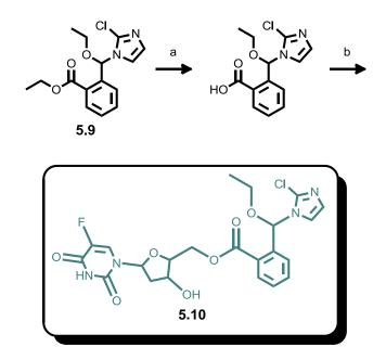
Figure 5.11 Schematic of the synthesis of 5.10. Reagents: a) LiOH in THF/water b) 5.6, 2M6NBA, DMAP, TEA, Microwave, 100 °C. 6% yield.
