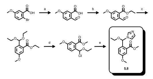
Figure 5.9 Schematic of the synthesis of 5.8. Reagents: a) n-BuLi, DMF, -78 °C, 51% yield, b) Etl and sodium carbonate in DMF, 52% yield, c) ethyl orthoformate, EtOH, TsOH, 88% yield, d) thionyl chloride, reflux, neat e) imidazole, NaH in THF, 30% yield over two steps.
