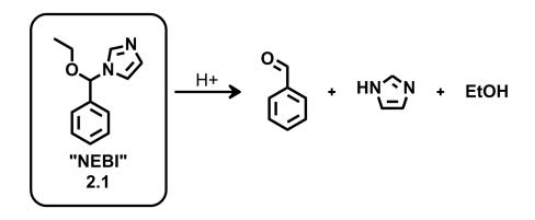
Figure 2.3 Hydrolysis of the NEBI gives benzaldehyde, imidazole and EtOH.
