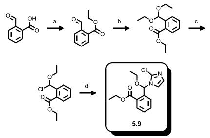
Figure 5.10 Schematic for the synthesis of 5.9. Reagents: a) Etl and potassium carbonate in DMF, 71% yield b) ethyl orthoformate, EtOH, TsOH, 67% yield, c) thionyl chloride, reflux neat d) 2-chloro-imidazole, NaH in THF, 60% yield over two steps.
