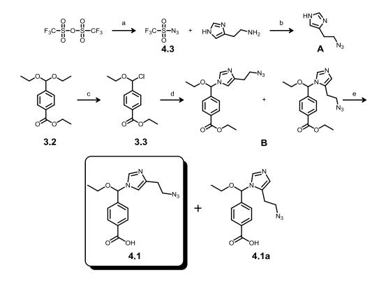
Figure 4.2 Synthetic scheme for bifunctional crosslinker para-Nethoxybenzylimidazole-azide-carboxylic acid 4.1. Reagents: a) sodium azide, DCM and water; b) potassium carbonate, copper sulfate, in DCM, MeOH, and water 53 % yield for two steps; c) acetyl chloride, thionyl chloride; d) A, NaH, in THF, 28% yield over two steps; e) lithium hydroxide, water and THF.
