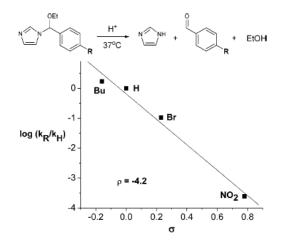
Figure 2.7 Linear Hammett correlation for the hydrolysis of 2.1-2.4 in 0.5 M MES buffered  $D_2O$  (pD = 5.5) at 37 °C, where R = n-butyl (Bu), H, Br, and  $NO_2$ .
