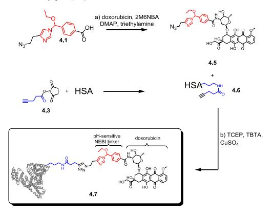
Figure 4.4 Conjugation of doxurbicin to HSA via a NEBI linker using click chemistry. TCEP = tris(2-carboxyethyl)phosphine, TBTA = tris-(benzyltriazolylmethyl)amine
