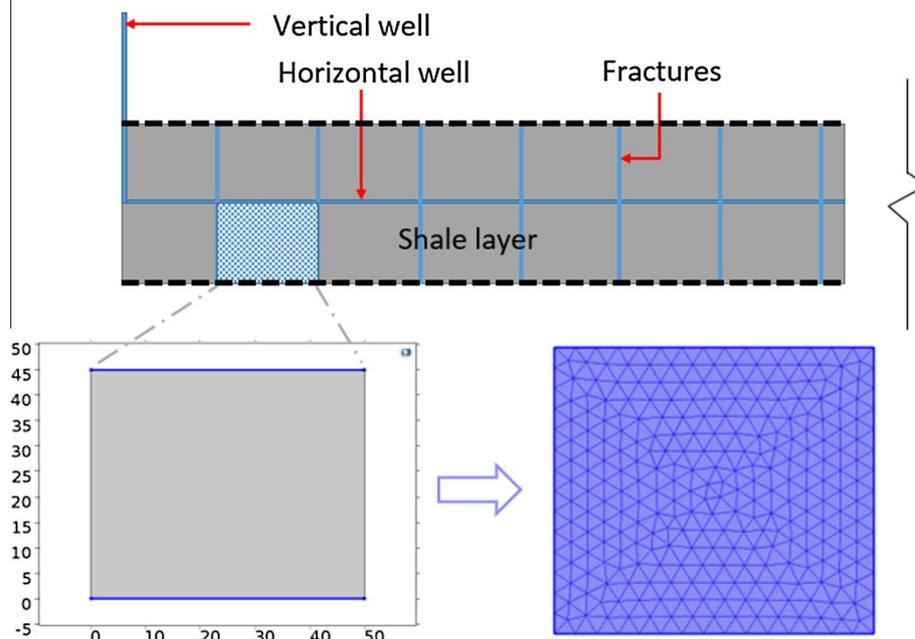
Fig. 3. Simplified geometrical model.
