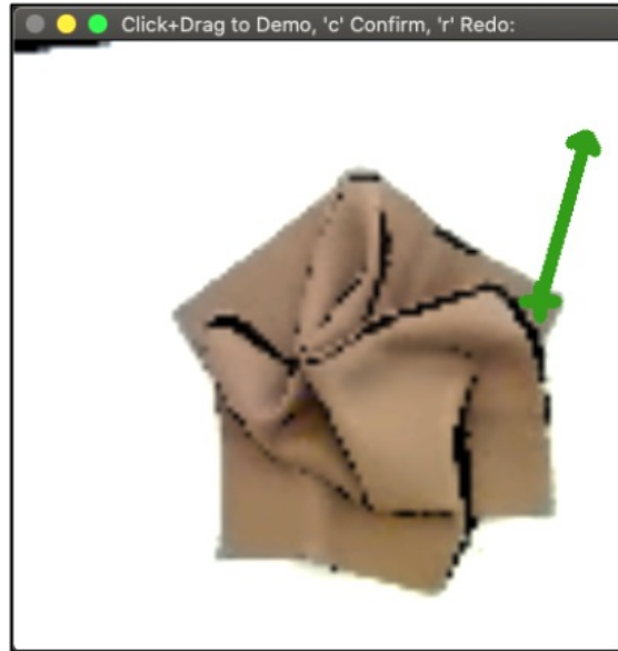
Figure A.3: The user interface for human interventions. The current observation of the fabric state from the robot's perspective is displayed, with an overlaid green arrow indicating the action the human has just specified.
