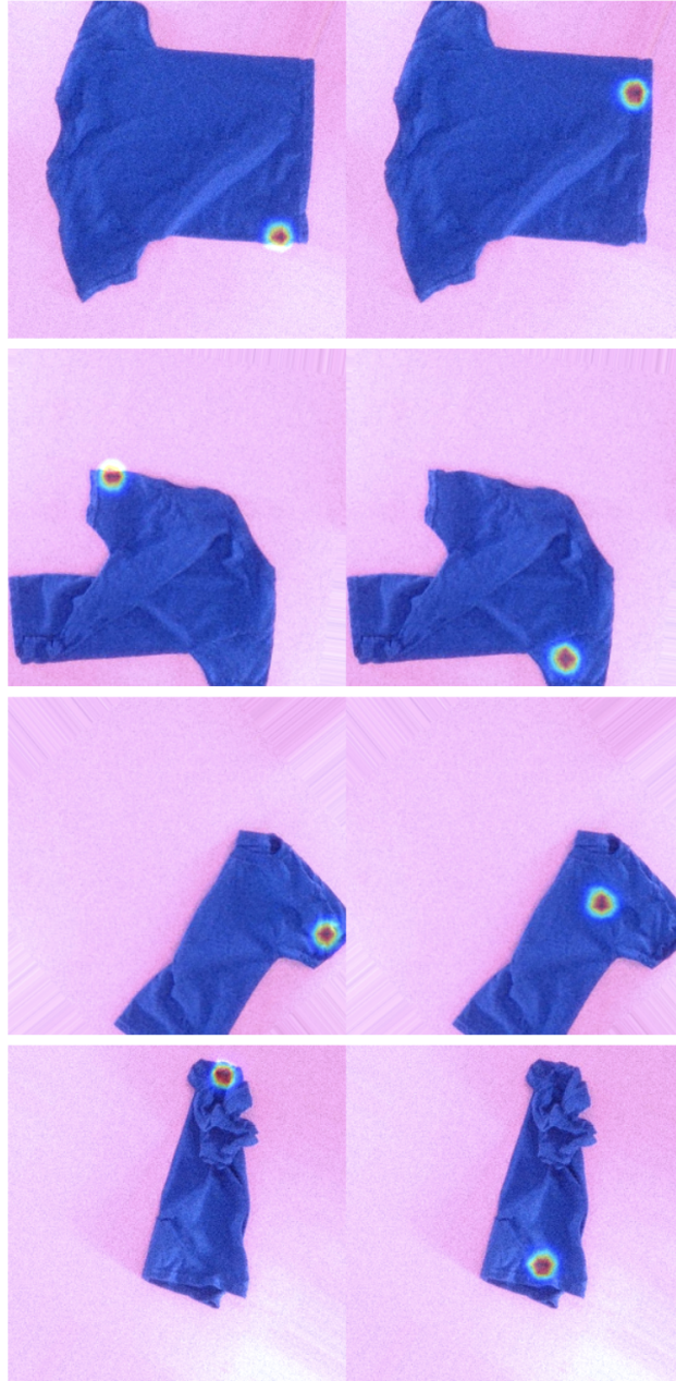
Figure E.2: LP_0LP_1 keypoint predictions on the test set (i.e., unseen affine transforms). Each row is a different data sample where the left image shows the predicted pick and the right shows the predicted place. The 4 steps together comprise a folding demonstration.
