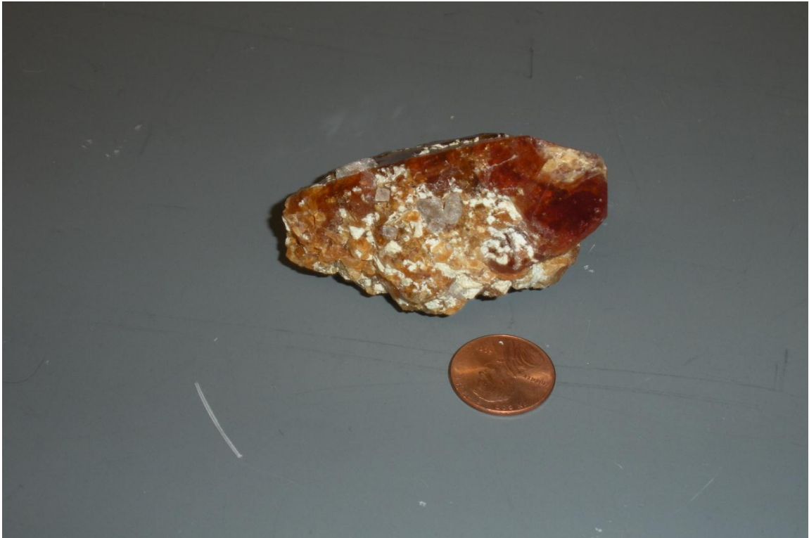
Figure 2. Some of the scheelite used for experiments shown in its original state before crushing and sorting. The grayish and white materials on the surface of the orange scheelite crystal are quartz and muscovite. Both were removed during sorting.
