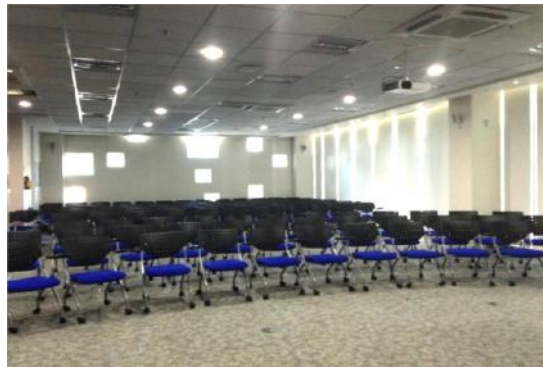
Left: picture of the underfloor air distribution outlets in the office spaces. Center: conference room with UFAD and ceiling-mounted split air system, with punched windows for diffused light. Right: the server room with a ceiling diffuser for ventilation and individual air conditioner for cooling.
