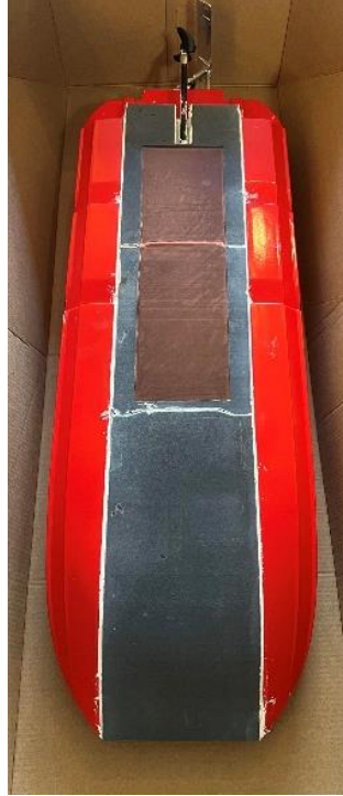
Figure 3.10: The double-sided tape with its orange plastic liner covers the recess, preventing water from permeating into the surface of the uncoated portion of the Nylon 12 sample holder plate.
