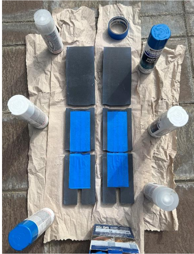
Figure 3.6: Spray-coating the Nylon 12 holder plates with NeverWet spray. The recess of the holder plate is covered so that it is not coated with NeverWet.
