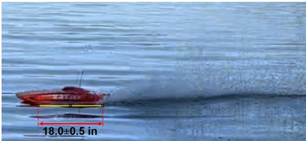
Figure 3.18: An image of the model boat traveling at 100% throttle, such that it acts as a planing hull. This image is uploaded to ImageJ software to determine visually (i.e., via pixel count) that the wetted length is approximately 18.0±0.5 inches.
