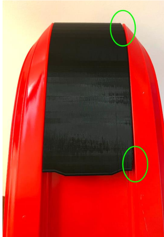
Figure 3.5: When printing the holder plate components using FDM 3D-printing, the warped shape of the component exposes gaps in the new hull design, as highlighted by the green circles.
