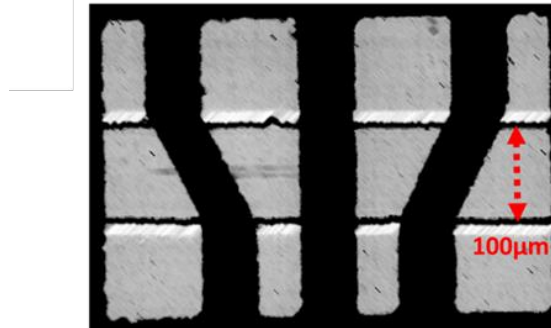
Figure 3.3 The image of the sensing area under CCD camera, indicating the uniform illumination is applied over the four slits to allow the incident light to be encoded.
