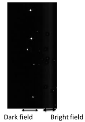
Figure 6.8 A snapshot of 15 \mu\text{m} polystyrene beads interrogated with the scattering-imaging-based cytometer platform, showing clear scattering images in the dark field and a bright band for self-contained verification. Due to the software setting, the brightfield imaging is shown in the downstream direction to align with the sliding direction.
