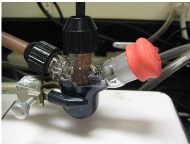
Figure 3.1 A double Clark electrode system reported by the Grotjahn group in 2011. One of the electrodes is submerged in the reaction mixture whereas the other is in the headspace.
