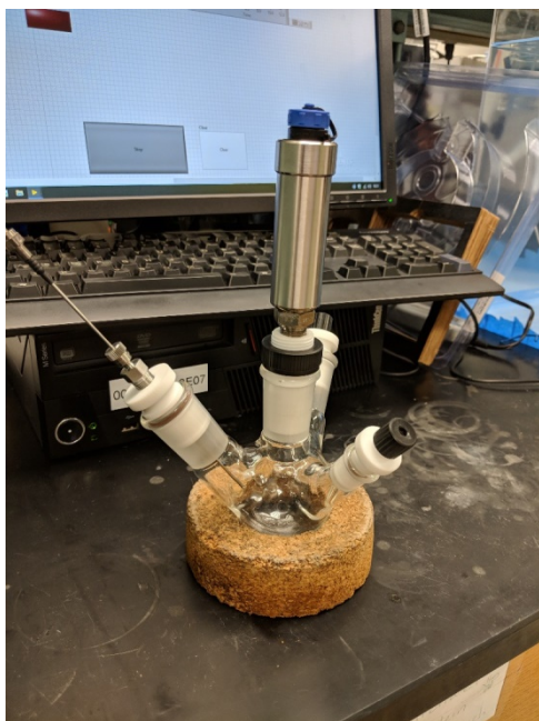
Figure 3. 2 An early attempt at cell design. We used off the shelf adapters and modified them to accommodate O-rings for extra sealing, but the cells still leaked.
