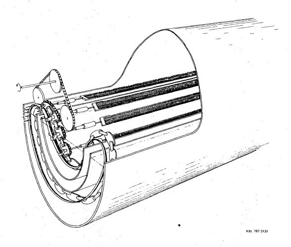
Fig. 1: Cutaway view of Cam-Track Nitinol engine concept. One end of the tank is shown, with concentric water baths, typical power elements, one of the pair of cam-tracks, and power take-off.
