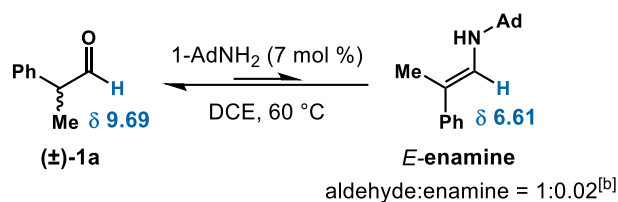
Figure 2.7 Enamine formation studies. [a] Reaction conditions: 1a (0.15 mmol, 1.0 equiv), 1-AdNH 2 (7 mol % or 1.0 equiv), DCE (0.2 mL). [b] Ratio determined by 1 H NMR analysis of a portion of unpurified reaction mixture. With 1.0 equiv of 1-AdNH 2 , aldehyde: enamine = 1:1.7.
