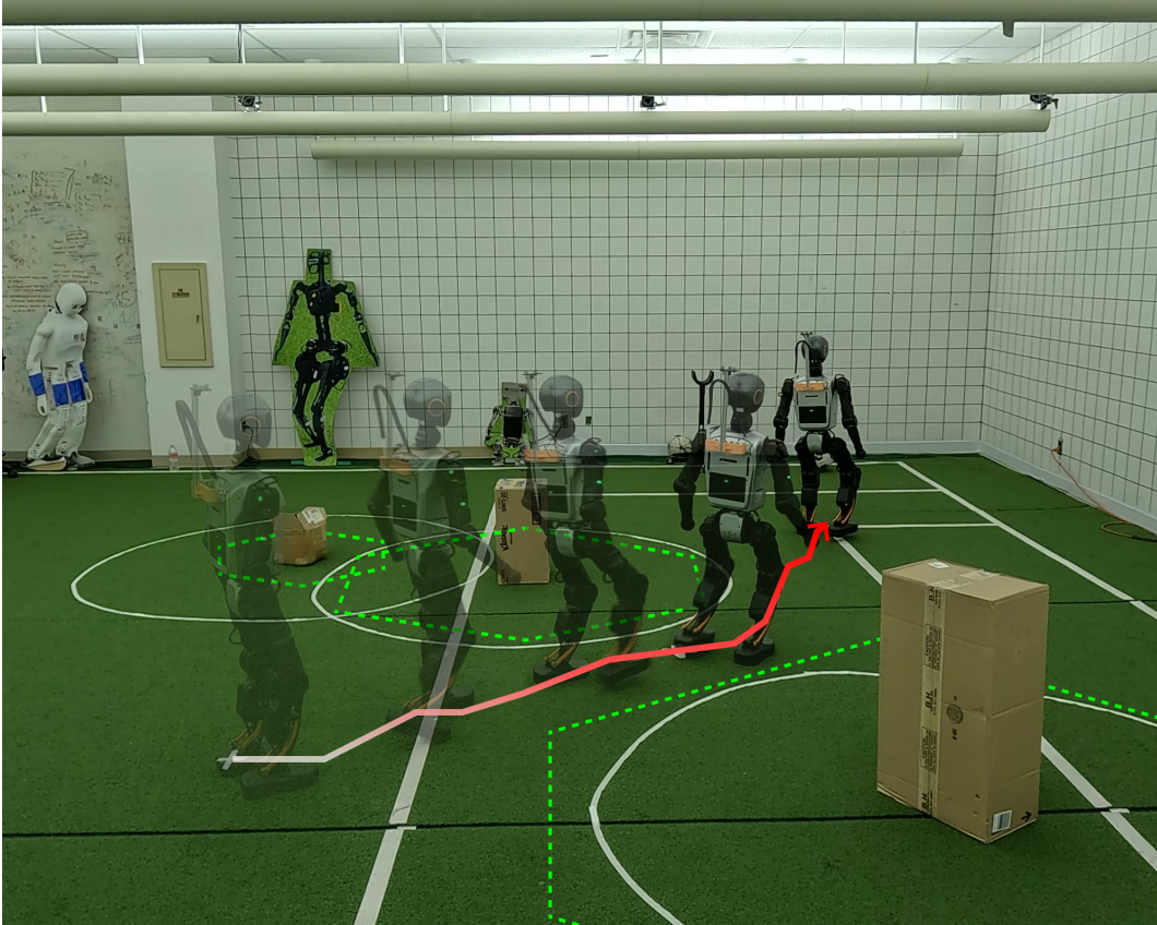
Figure 1.1: The RAVEN framework deployed on the T1 Booster biped navigating among obstacles. Hexagons indicate the adaptive obstacle inflation regions whose radii are determined by the RL meta-policy to account for control delays and tracking uncertainties.
