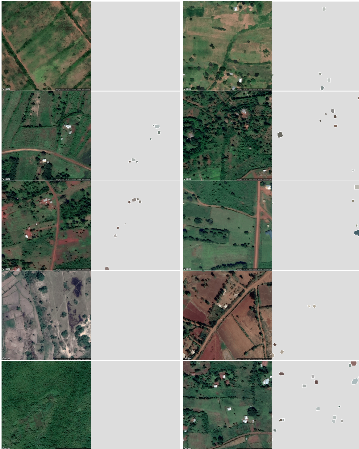
Figure A.2: Ten randomly sampled pairs of input images and deep learning predictions. Ten images are randomly sampled from all the input satellite images in the GiveDirectly study area. Each predicted building is outlined in white and filled with the “representative” roof color.
