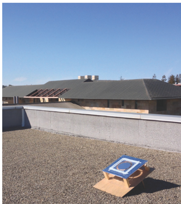
Figure 36. Outdoor test of a daytime radiative cooling surface. A test stand that insulates and minimizes parasitic heat gain is essential to maximize performance. A unique feature of radiative cooling experiments is the need to perform tests outdoors.
