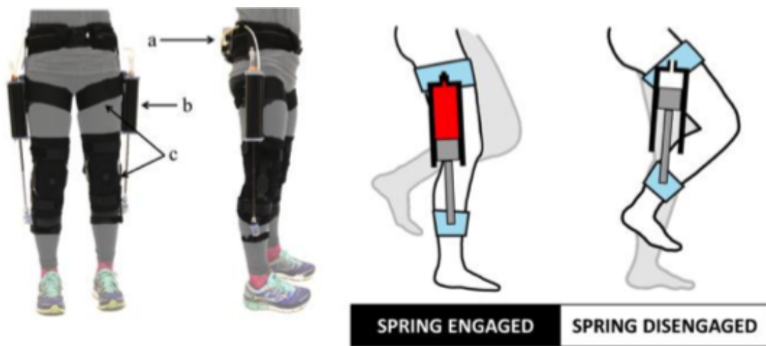
Figure 2.6: Quasi-passive knee exoskeleton that varies spring levels by the timing of engagement/disengagement to accommodate for mechanical performance and reliability [8].
