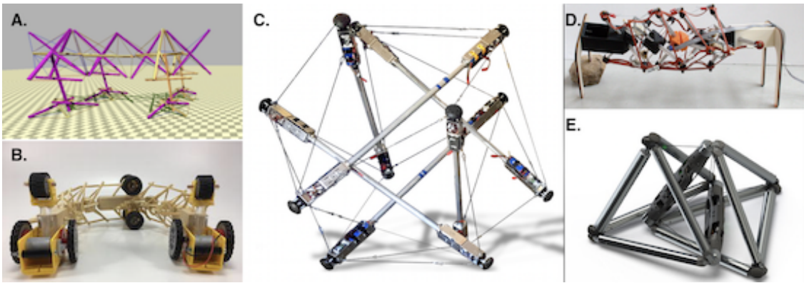
Figure 2.8: Tensegrity Robotics - A: Vertebra-inspired quadruped [12]. B: Wheeled spine-inspired robot (WTR) [13]. C: Tensegrity SUPERBall [14]. D: Laika quadruped robot [15]. E: Duct climbing robot (DUCTT) [16]
