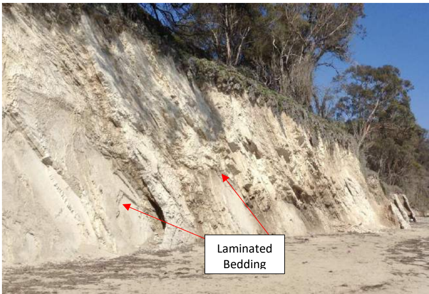
Figure 10. Image of the upper Monterey. Note the steep bedding dip and the laminate like nature of failure. Photo: Klath 2015, Goleta beach (east end).
