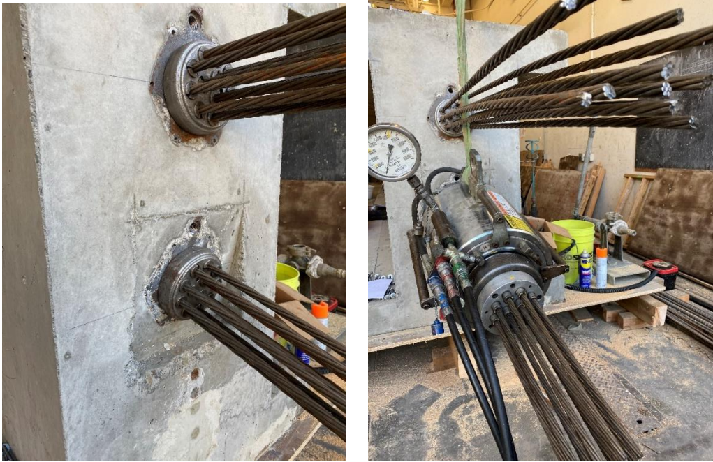
Figure 2.22: Post-tensioning of specimen #2
