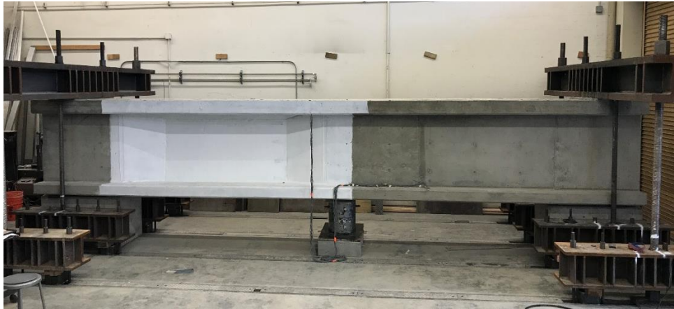
Figure 2.23: Specimen #2 mounted on end blocks with reaction system installed
