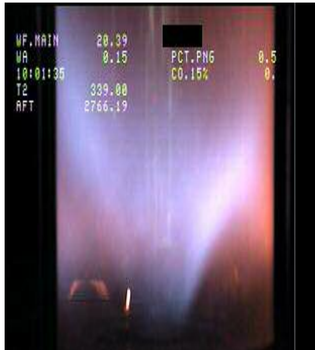
Figure 5.2: Stable flame conditions ( W_f=20.39 lbs/hour, W_a=0.15 lbs/s and T_{adiabatic}=2766^\circ\text{F} ).
