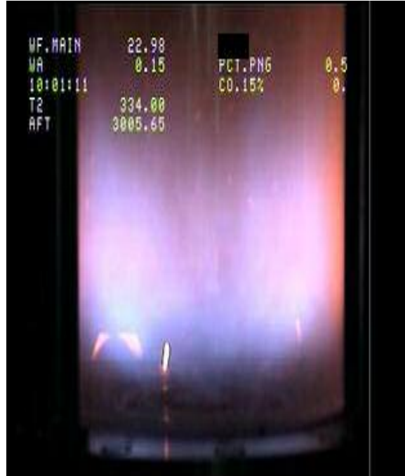
Figure 5.3: Flame oscillation at 250 Hz ( W_f=22.98 lbs/hour, W_a=0.15 lbs/s and T_{\text{adiabatic}}=3005^\circ\text{F} ).
