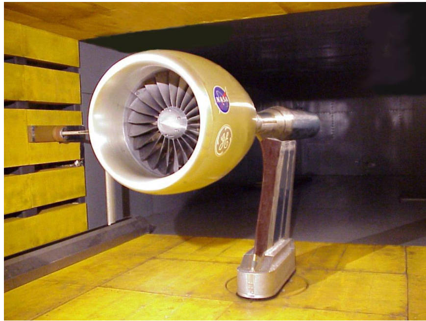
Figure A.1: 22 inch scale model of the Source Diagnostic Test (SDT) model fan installed in the 9-ft by 15-ft low speed wind tunnel at NASA Glenn from TM 2008-215415.
