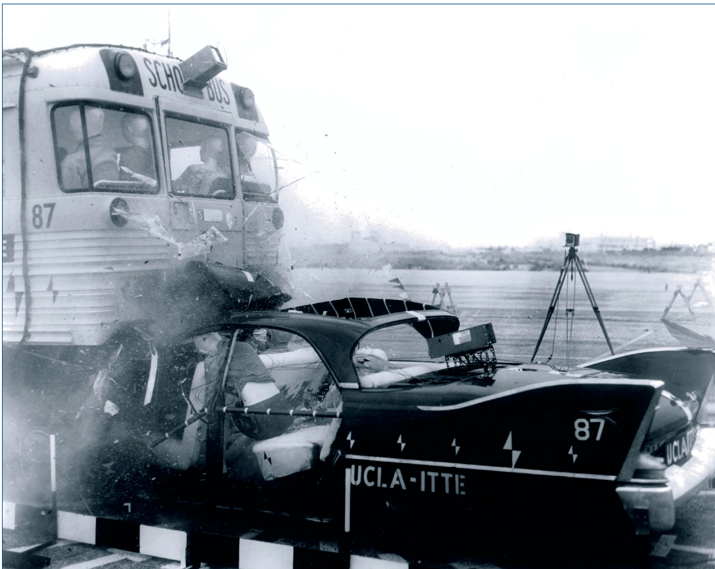
The Institute for Transportation and Traffic Engineering conducted more than 100 car and bus crash tests staged at an abandoned air strip at the U.S. Naval Station in Long Beach. Credit: UCLA Samueli School of Engineering.
