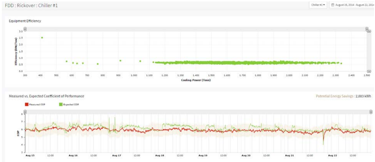
Figure 10. Screen shot of the chiller efficiency fault detection and diagnostic features in the PlantInsight tool for a fault-free period of operation
