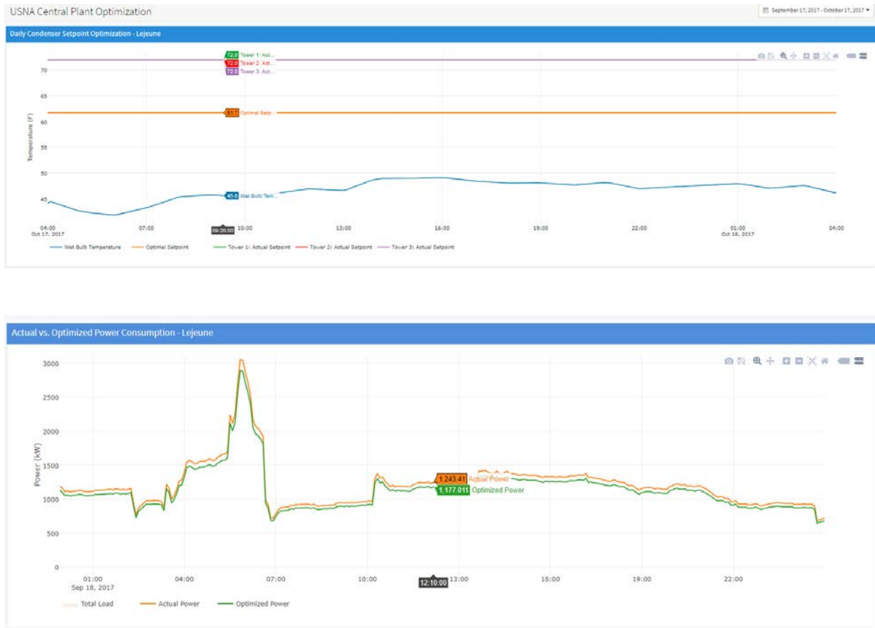
Figure 9. Screen shots of the condenser water temperature setpoint optimization features in PlantInsight: (Top) Optimal and conventional condenser water setpoints with predicted wet bulb temperature. (Bottom) Measured and predicted optimal power.
