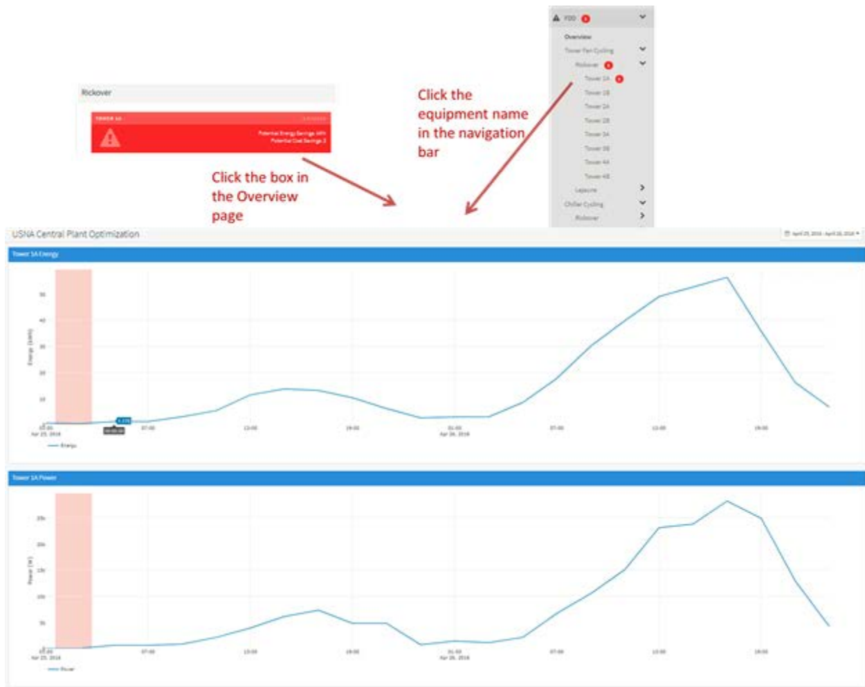
Figure F- 13. The equipment-specific fault drill-down page
