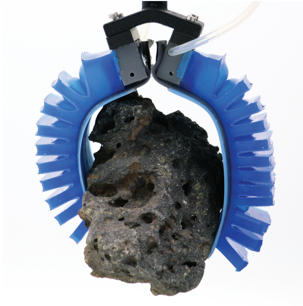
Figure 2.2: Active fingers allow for grasps on objects that do not typically support gecko-inspired adhesives. In many cases, the gecko elastomer actuator gripper does not depend on adhesion, but is enhanced by it. On dusty, irregular, or porous objects where adhesive performance is low, gecko elastomer actuator grippers still utilize force closure. (Mass of rock 150.1 g)
