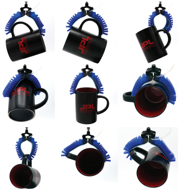
Figure 2.12: Elastomer actuator grippers with gecko-inspired adhesives are capable of a wide range of stable grasps. Gecko-inspired adhesives enhance grasp choice by reducing the minimum chamber pressure for a stable grasp and by increasing grip strength at a given chamber pressure. Gecko-inspired adhesives also enable grasps that are not possible through load-controlled friction.
