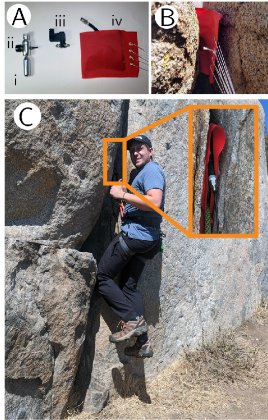
Figure 4.8: An inflatable anchor that is light weight and easily positioned. (A) Components of the anchoring system include CO 2 cartridge (i), pressure regulator (ii), valve (iii), and inflatable pouch (iv). (B) The pouch is easily placed in a wide range of channels when deflated, and conforms to arbitrary surfaces to provide holding force when inflated. (C) We demonstrate the capability of these anchors by holding a human ( < 700 N load) at 105 kPa of internal pressure using a microspine interface.
