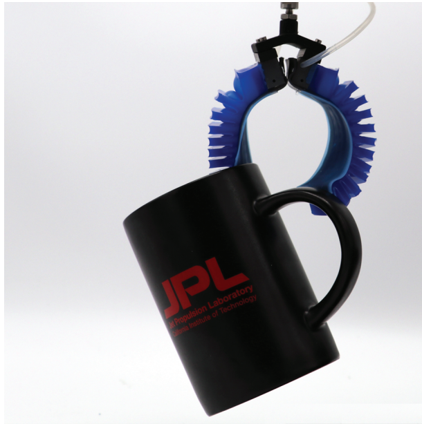
Figure 2.1: Gecko elastomer actuator grippers can achieve versatile grasps on complex shapes. The gripper passively deformed and reached this stable grasp to react a 20 degree twist applied to the base of the mug. (Mass of mug 397.7 grams).
