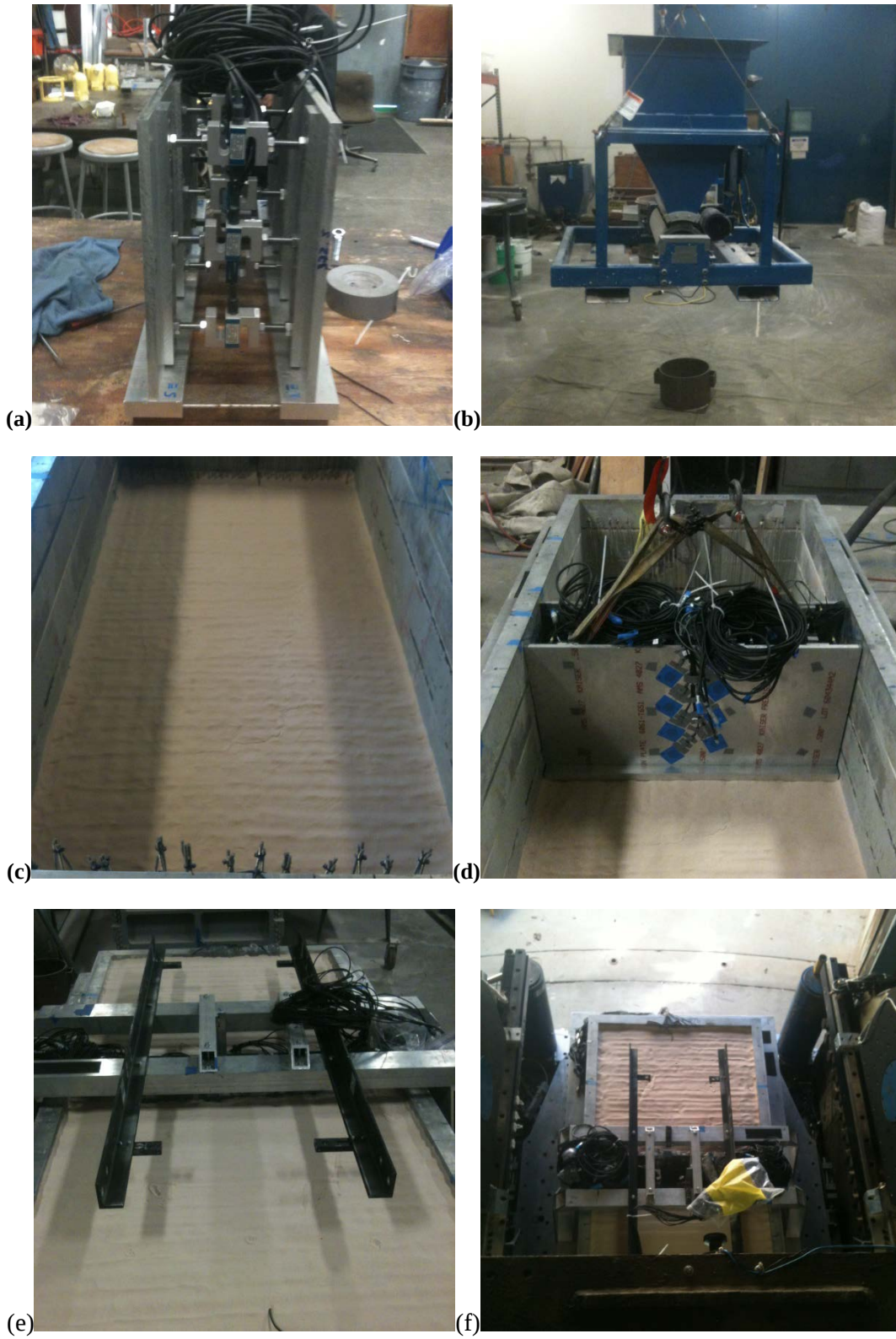
Figure 3.7: Model construction (a) wall construction, (b) pluviator calibration, (c) placing sand, (d) placing structure, (e) fitting aluminum frame, (f) model on arm
