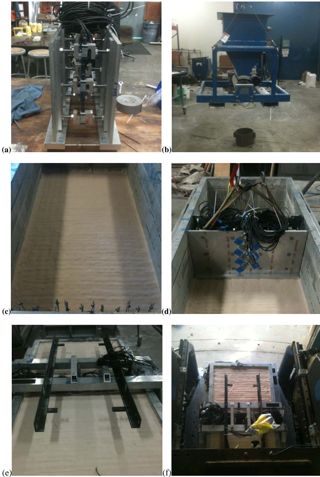
Figure 3.7: Model construction (a) wall construction, (b) pluviation calibration, (c) placing sand, (d) placing structure, (e) fitting aluminum frame, (f) model on arm
