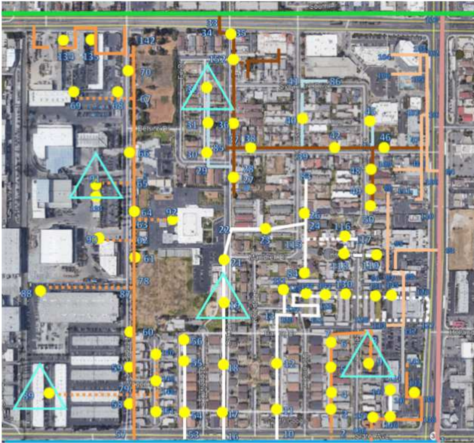
Figure 13 Selection of nodes that serves as growing points are marked in blue triangles. Note that although each islanded scenario has same starting points to form islands, the eventual island formation may differ as the imbalance between electric demand and supply changes.
