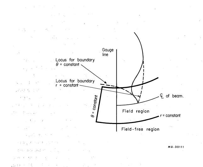
Fig. 5. Qualitative illustration of composition of the  $\theta_t$  contour line from two loci corresponding respectively to emergence of the beam through end or side of the magnetic field.
