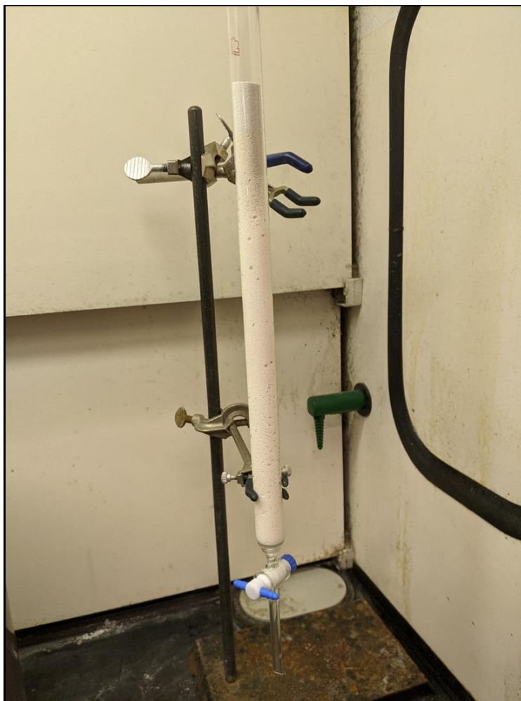
Figure 27- The ion-resin exchange column shown above was used to purify the botryococcene polyol. The resin used (Amberlite IRA 743) was specifically chosen for borane complex removal. Vacuum pressure was not required but can be used for accelerated filtration.
