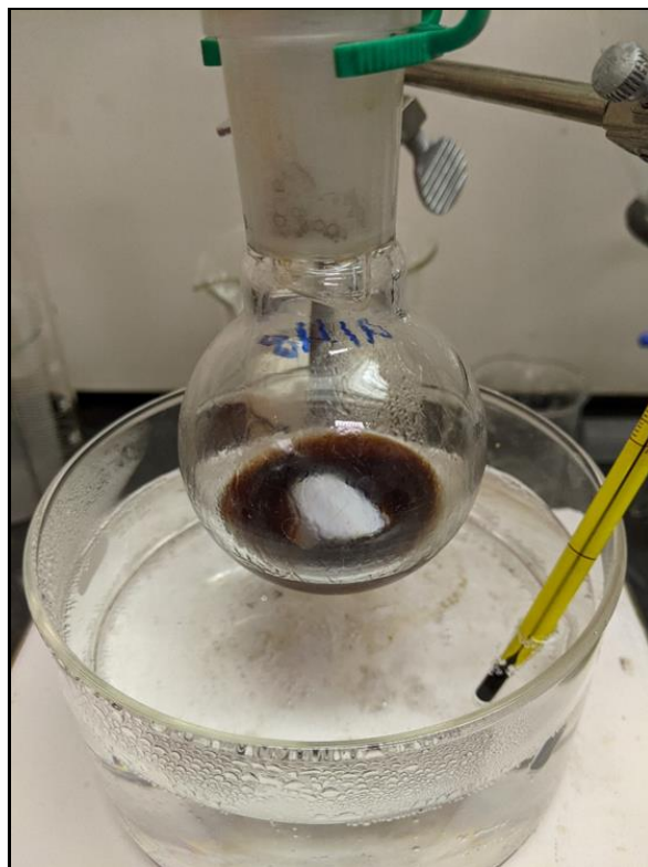
Figure 26- The sulfuric acid catalyst will turn the epoxide mixture a chestnut brown color; this type of color change was not observed with other acid catalysts. The brown mixture turned clear upon the addition of hydrogen peroxide.
