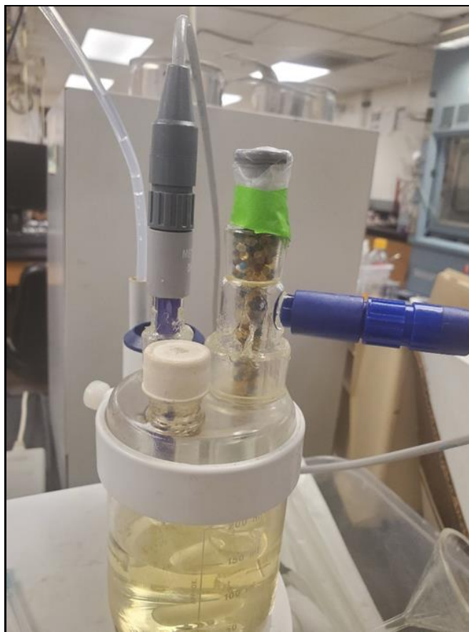
Figure 19- The Karl Fisher cell is a highly specialized piece of glassware that can hold up to 200 mL of Hydranal Coulomat A with the probes in place. The gray probe measures potential and the blue probe is the generator electrode. The injection site is sealed with a rubber septa (white).
