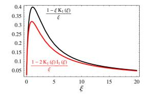
FIG. 1: The black curve is proportional to the SC impedance relative to the on-axis longitudinal electric field for a uniform beam with circular cross-section, see Eq. (8). The red curve is proportional the SC impedance averaged over the transverse density of the same beam, see Eq. (12). The variable  $\xi$  is defined as  $\xi = kr_b/\gamma$ .
