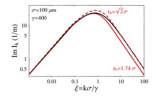
FIG. 3: The (absolute value of the) quantity  $I_k$  as a function of  $\xi = k\sigma/\gamma$  for an axis-symmetric gaussian beam with transverse rms sizes  $\sigma$  [black curve, see Eq. (15)] is contrasted with that of a beam with uniform transverse density for two choices of the radius  $r_b$  (red curves).
