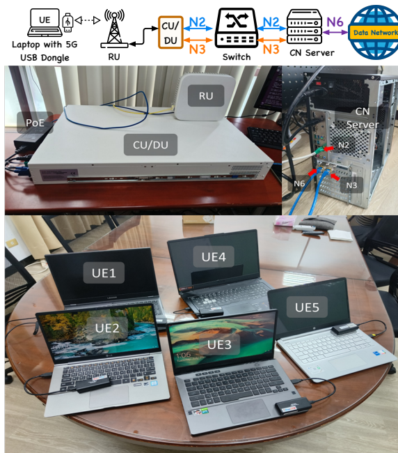
Figure 7.5: (Top) The logical topology, and (Bottom) a snapshot of commercial testbed setup in L 2 5GC+. RU: Radio Unit; DU: Distributed Unit; CU: Central Unit; CN: Core Network; PoE: Power over Ethernet; 5 laptops as UEs with 5G dongles
