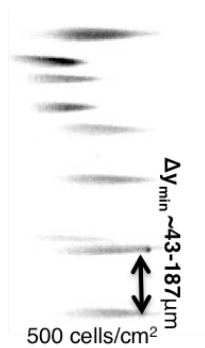
Figure 3-8. Lamin A/C peaks are resolved laterally at a low (500 cells/cm 2 ) cell density. To pattern single cells that were resolved laterally (perpendicular to the IEF axis), we used the characteristic diffusion equation ( \tau \sim X^2/D ) to determine the cell-to-cell spacing for minimally resolved lamin A/C peaks. We used already reported lamin A/C diffusion coefficients, 3 and factored in in-gel diffusivity of proteins in a 6%T, 3.3%C gel. 4 Given our 390 s assay time, we estimated cells needed to be spaced 43-187 \mu\text{m} (depending on which diffusivity used) apart. For the 500 cells/cm 2 seeding density, the peaks were spaced 74 \pm 71 \mu\text{m} (mean \pm s.d., n = 38 cells) apart. Thus, most (~70%) focused IEF protein peaks are minimally resolved and thus can be indexed back to a single adherent cell.
