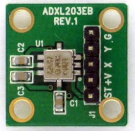
Figure A.4: Accelerometer with Evaluation Board [2] [1].
