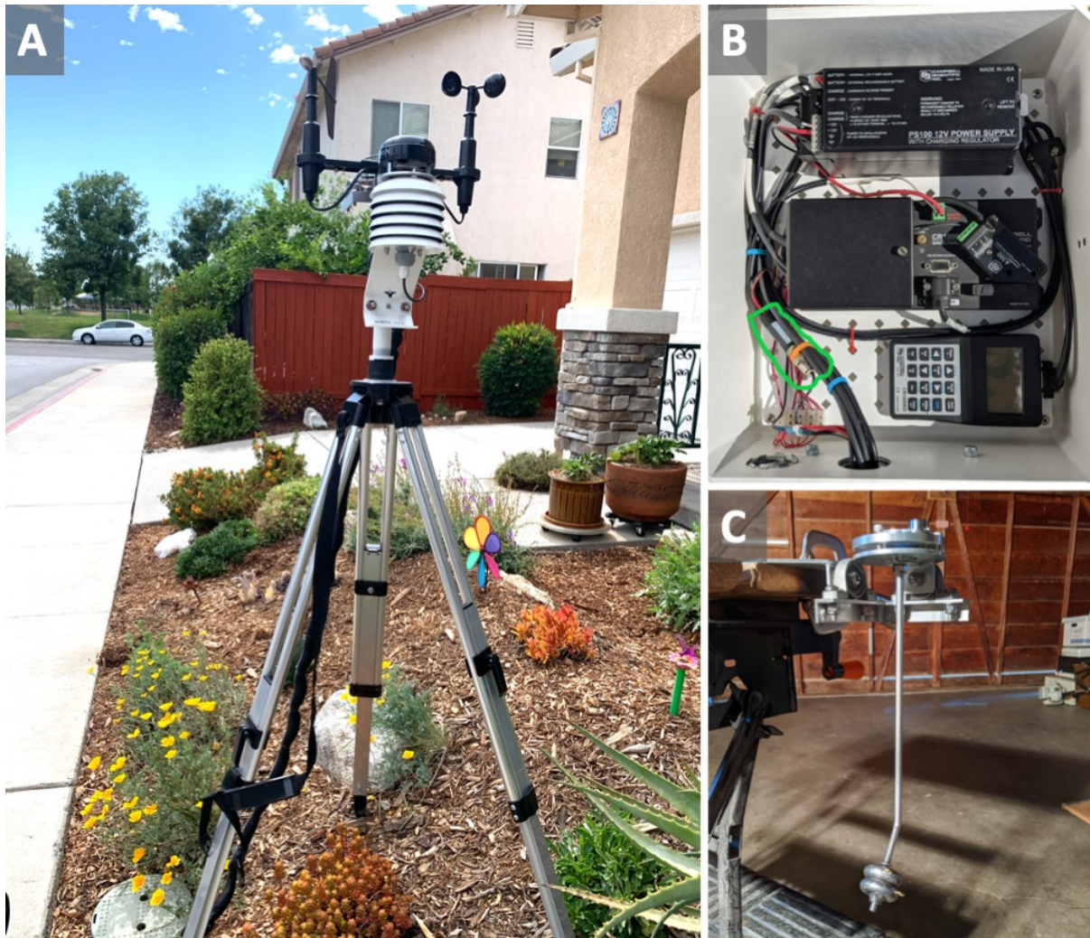
Figure S1. Custom-built micrometeorological station. A) Station at human-height in a sampled yard. Image shows the station on an adjustable tripod, with the aspirated temperature and relative humidity sensor, wind vane, and three cup anemometer all visible. Note, the pyranometer is present, but not visible on the other side of the station. B) Interior of the datalogger box, including signal converter and the CR1000X datalogger. C) Hand-made and self-levelling pyranometer mount with a gimbal.
