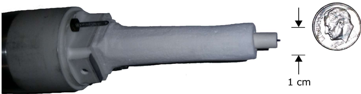
Figure 3.7: Picture of emissive probe and the relative size of the measuring probe tip and the support structure.
