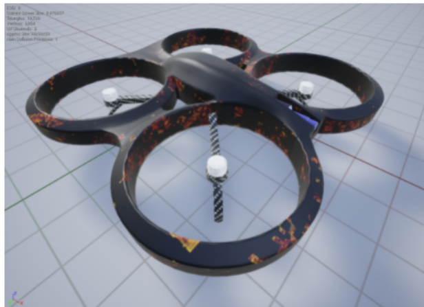
FIGURE 3.4. 1 Meter Wide Racing Drone Model from Airsim. The Airsim engine includes all the physics component to the racing drone.
